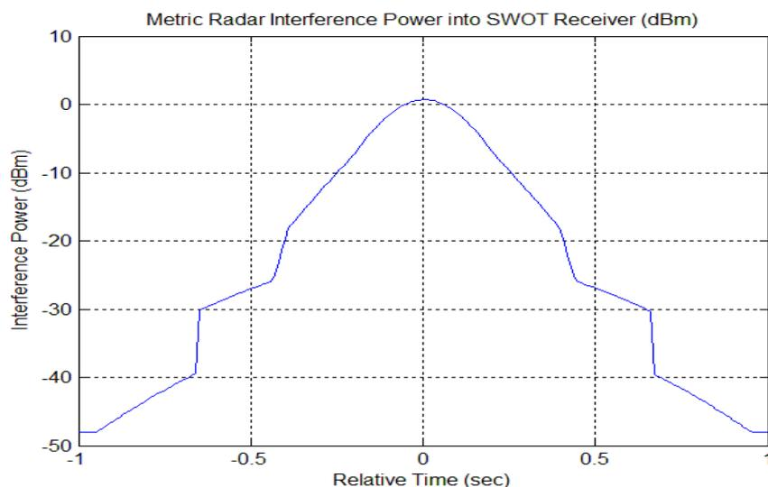
In Figure 8, the absolute worst case peak interference power is +0.67 dBm. The duration for the -3 dB power points is 0.24 seconds and the duration of the -10 dB power points is 0.5 seconds.
