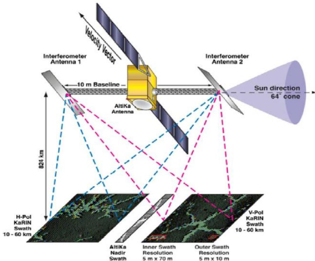
The 35.5-36.0 GHz InSAR transmits linear FM pulses with 1300 MHz bandwidth centered at 35.35 GHz with a pulse repetition rate approximately at 4400 Hz per antenna. The signal is horizontally and vertically polarized at both transmission and reception. The significant parameters for the InSAR are given in Table 1.
